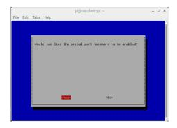
Finally, our UART is enabled for Serial Communication on RX and TX pin of Raspberry Pi.
