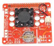
6. Screw the 4 x 7mm spacers to the rear of the PCB with the provided nuts as per the image below:
