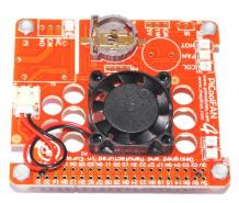
7. Fit your **PiCoolFAN4** on to the Raspberry Pi 4. For basic usage there is no need for any software installation.
